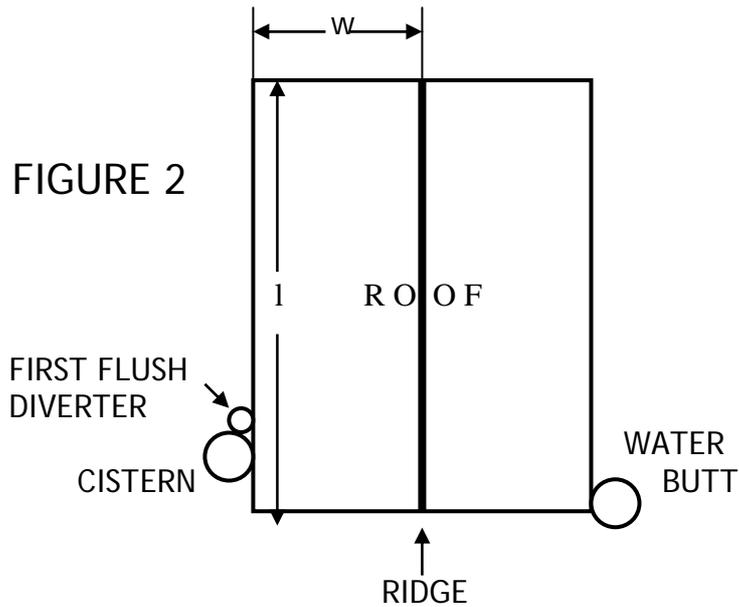
The mean annual rainfall (mar) for Worcestershire, U.K. is about 0.67 m. The efficiency of collection (e) for a rough-tiled surface is about 80% (a corrugated iron roof would be over 90%). The roof (collection area) is 9.3 m long and 3.5 m wide.
